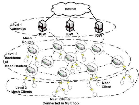
Figure 1. The hierarchical architecture of a WMN
