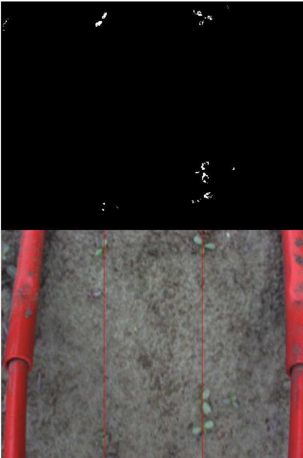
Figure 14: Illustration of the Belgian chicory results. Above: segmentation results of one camera image. Below: original camera image with superimposed the two estimated crop row positions (red).
