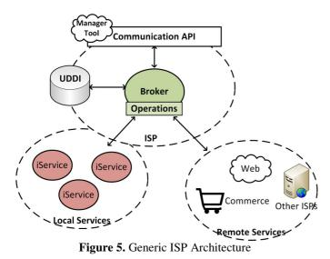
The front-end layer is the only way clients can access the ISP. This layer offers ways to publish and access application service; and an intermediary service (broker) who acts generically offering a standard interface (form of communication) for the communication between applications and services manages the access.
