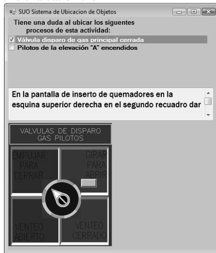
Figure 3. SUO system includes both data: (1) task to perform and their sequence (upper part) from the task model and (2) recommendations and graphic components (middle and lower part) from the user model.
