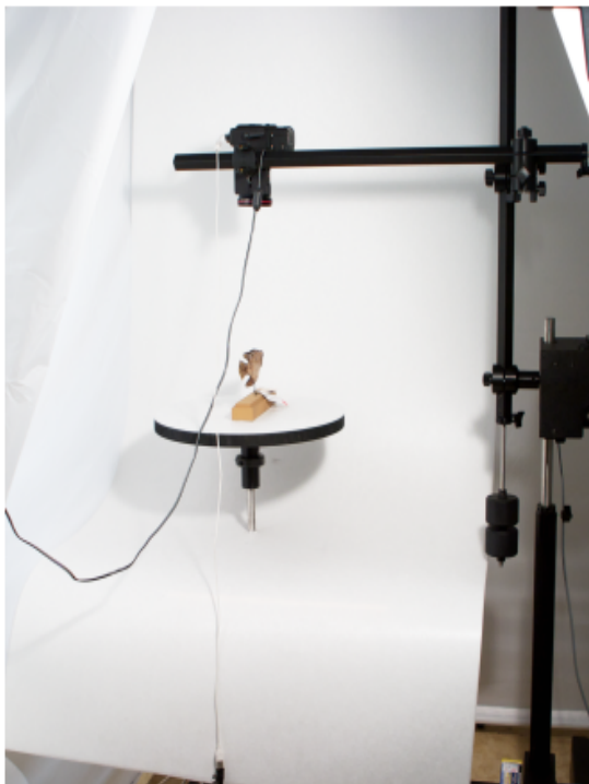
Figure 2. Motion-Control-Camera setup with object on turntable
