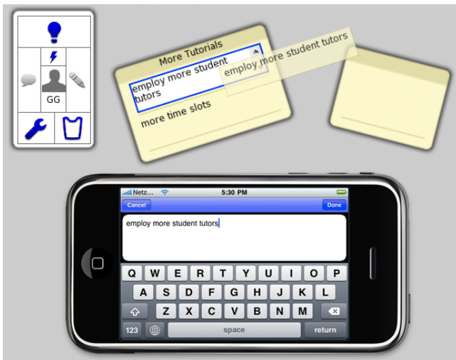
Figure 3: Tabletop widgets and iPhone interface. Clockwise from top left: control widget, idea card with two aspects (top one being moved), empty idea card, coupled iPhone app for text entry.
