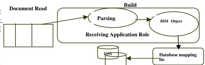
Figure 4.5: Message parsing and mapping fields to the database
