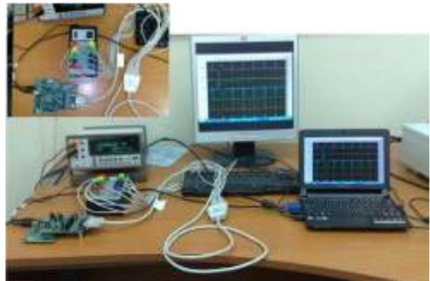
Figure 2. Experimental setup used in this work. Inset shows top view of connections for the simulator and the data acquisition modules.
