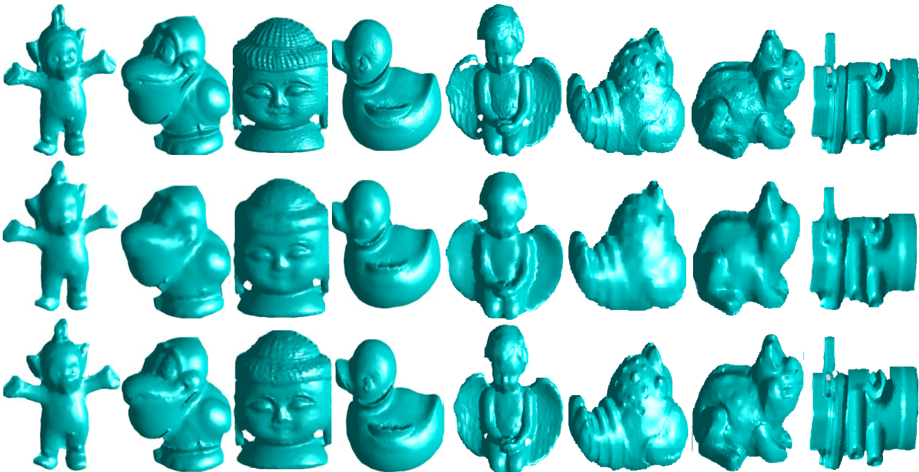
Figure. 7: Simplification by using QSim and SSim and simplification rate 90% on tubby, bird, buddha, duck, angel, lobster, frog and valve. Top column: Original; Middle column QSim; Bottom column: SSim
