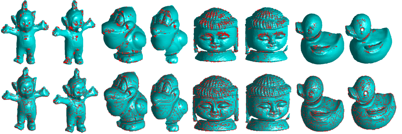
Figure 5: Points sampled on model tubby1-2, bird1-2, buddha1-2 and duck1-2 with simplification rate 90%. Top row: local points sampled. Bottom row: combined global and local sampled points in an appropriate combination rate.
