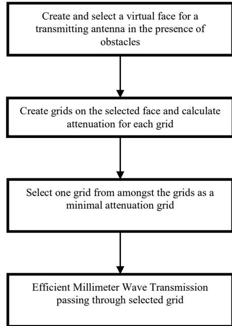
Figure 1. 5G mmWave grid selection for 5G transmitting antenna
