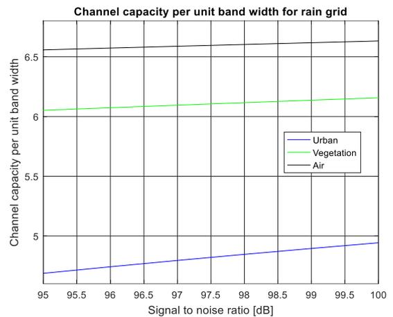
**Figure 18.** 5G mmWave channel capacity in rain season for 28 GHz
