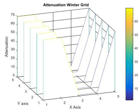
**Figure 19.** 5G mmWave grids attenuation values for atmospheric, vegetation in-leaf and building in winter season for 28 GHz.
