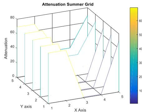
**Figure 15.** 5G mmWave grids attenuation values for atmospheric, vegetation in-leaf and building in summer season for 28 GHz.
