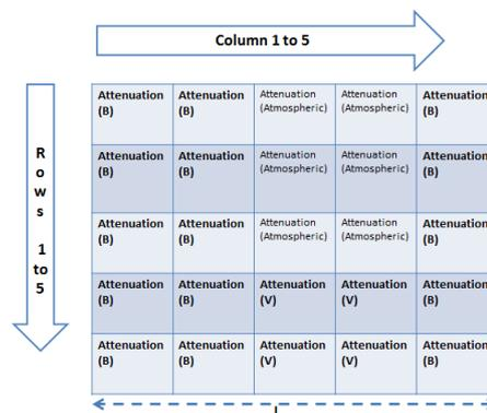
**Figure 5.** 5G mmWave grid with type of attenuations for DTU; having atmospheric, vegetation and building area
