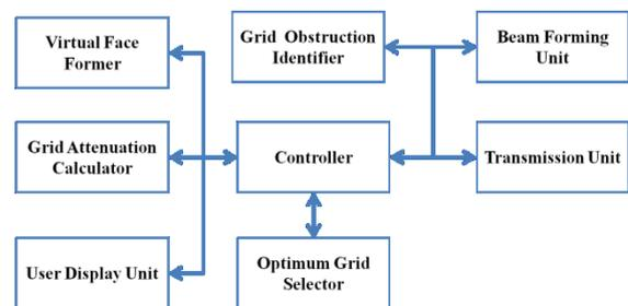
Figure 2. 5G mmWave intelligent grid selection and obstacle avoidance system
