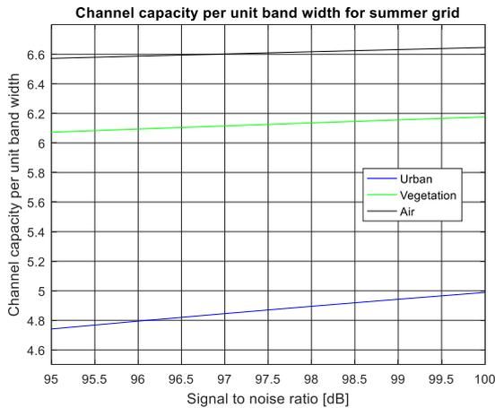
**Figure 16.** 5G mmWave channel capacity in summer season for 28 GHz.
