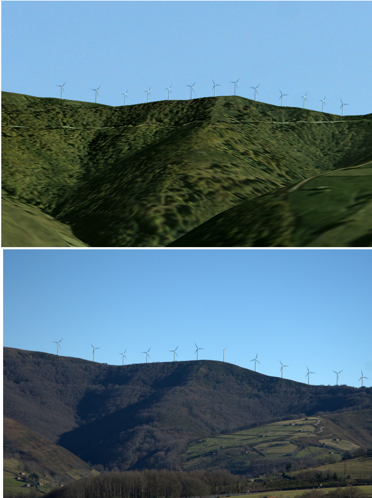
Figure 8: (top) Realistic visualization of a wind farm project taken from the Target and Camera points calculated by MOYSES. (bottom) Photograph taken from the same points referenced in UTM on site
