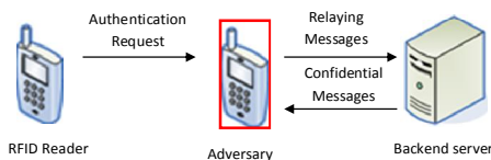
Figure 3. The example of an impersonation attack
