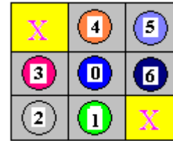
Figure 3. Distribution of 7 pixels constructed from rectangular pixels
